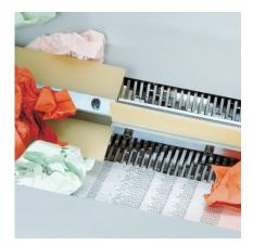
**BULK PAPER SHREDDING** Special rotating paddles are used to feed bulky materials into the cutting unit.
